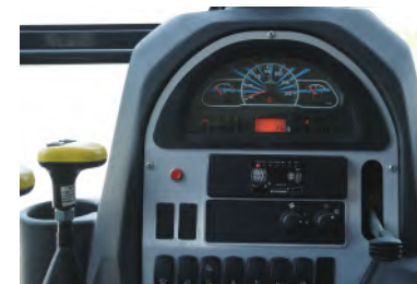
Multifunctional Single Instrument Cluster Panel With Night Glow Buttons.
